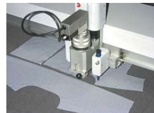
Cutting and marking tool head with oscillating tool
