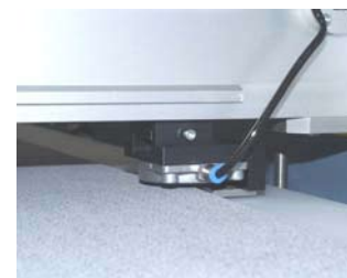
special feeding clamps grant an accurate material feeding
