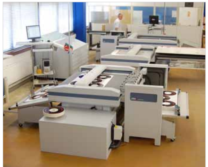
Production facility with the Zünd M-800 Cutter and Sheet Feeder.
